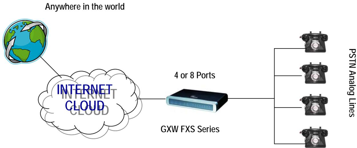
FXS Gateway acts as a 'virtual office', connecting analog lines directly to the gateway
