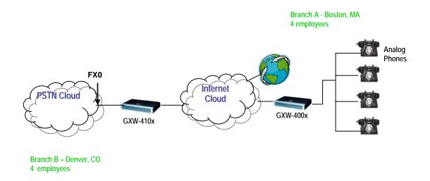
If you setup resembles the one in this diagram, you need to configure the SIP Server field to be the IP address of the other gateway (i.e. configure the IP address of GXW400x gateway to be the SIP Server for the GXW410x gateway and vice versa). <u>Please be sure you set SIP Registration to No.</u>
