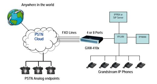
For incoming calls from the PSTN analog endpoints to the GXW410x gateway, the device will auto forward each call to a configured IP extension. The SIP Server can then route the call based on its own configuration or IVR system.
